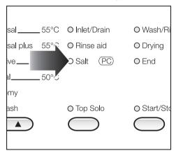
The indicator or check light marked "Salt PC" is used as the interface for this programming.
